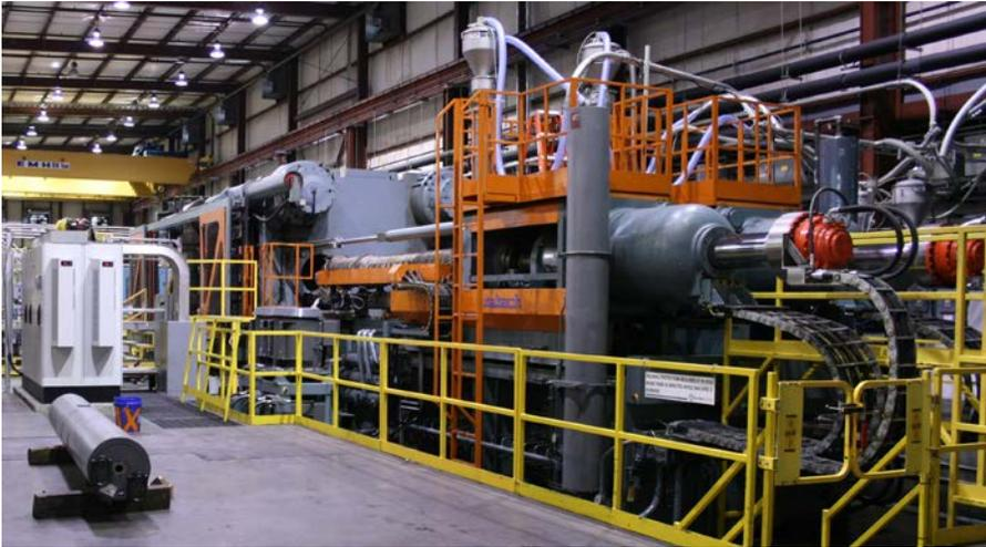
The heart of the retrofit to the Italtech is the B&R PC2100 which includes a 15" touchscreen controller. This system interfaces to every component of the press and ancillary equipment while monitoring everything from pressure and temperature to flow rates. "One of the great benefits of the new control system is the ability to monitor, support and upgrade it remotely," said Kitchen.
