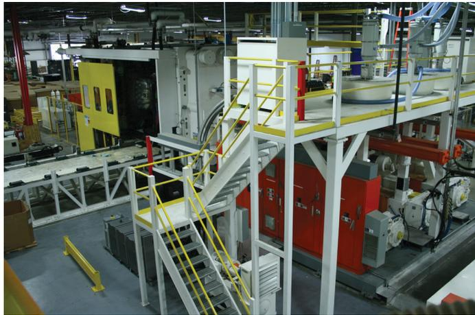
The custom press was designed specifically to produce large septic and potable water tanks – up to 1,787 gallons - at Infiltrator’s Winchester, Kentucky plant. Each polypropylene tank half measures up to 15 feet long and weighs in at an incredible 245 pounds. Infiltrator produces the tanks in halves that nest together to facilitate efficient shipping.
